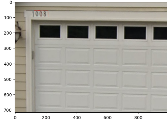
Figure 3: Example of another failure of the algorithm. Not all digits are detected within an image. This could be due to poor MSER performance or too strict of geometric filtering. This issue pertains to the recall criterion.
