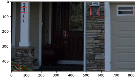
Figure 2: Example of one failure of the algorithm. Vertical squares are not handled correctly in this algorithm. Also, one of the door elements was classified as a "0" and one of the actual digits was filtered by the CNN threshold. The result of this classification was "3320".
